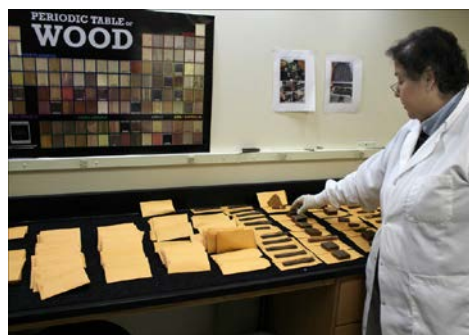
A forensic scientist prepares CITES protected wood samples for anatomical analysis. Credit: USFWS
